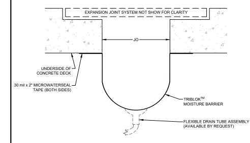
TGS Series Gutter System Sizes 300 through 2400 (Slab-to-Slab)
