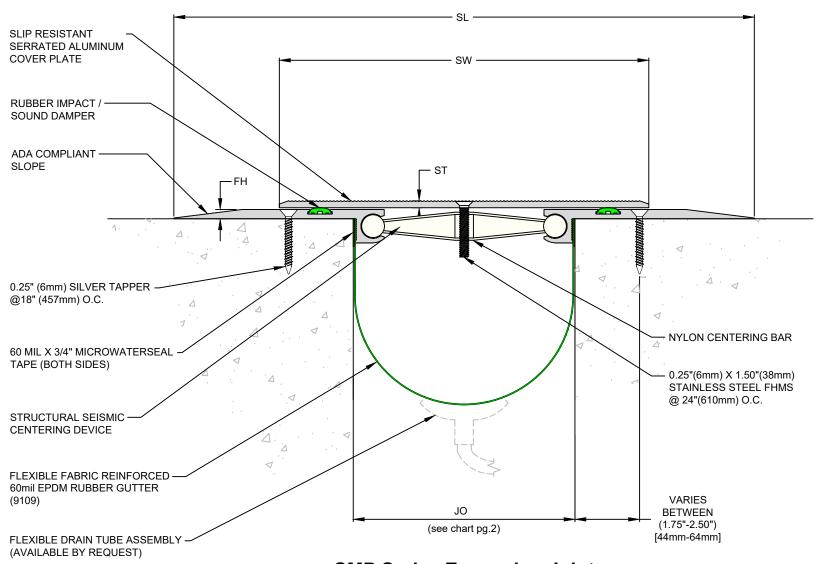
**SMP Series Expansion Joint** Sizes 400 through 1200 (Slab-to-Slab)
