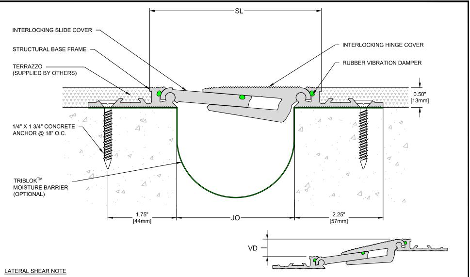
THE SIH ACCOMMODATES PROJECT SPECIFIC LATERAL SHEAR REQUIREMENTS. CONTACT MM SYSTEMS FOR ADDITIONAL INFORMATION.
