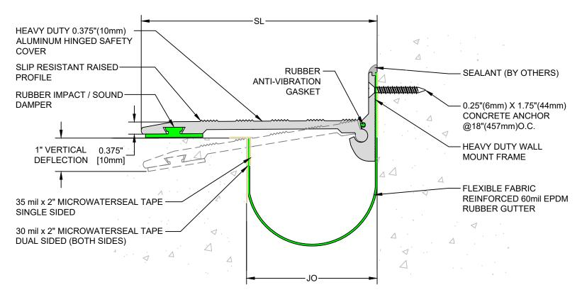
**HSC-C Series Expansion Joint** Sizes 200 through 1200 (Slab-to-Wall)
