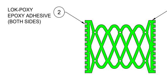
**ELASTOPRENE RUBBER** WATERPROOFING SEAL
