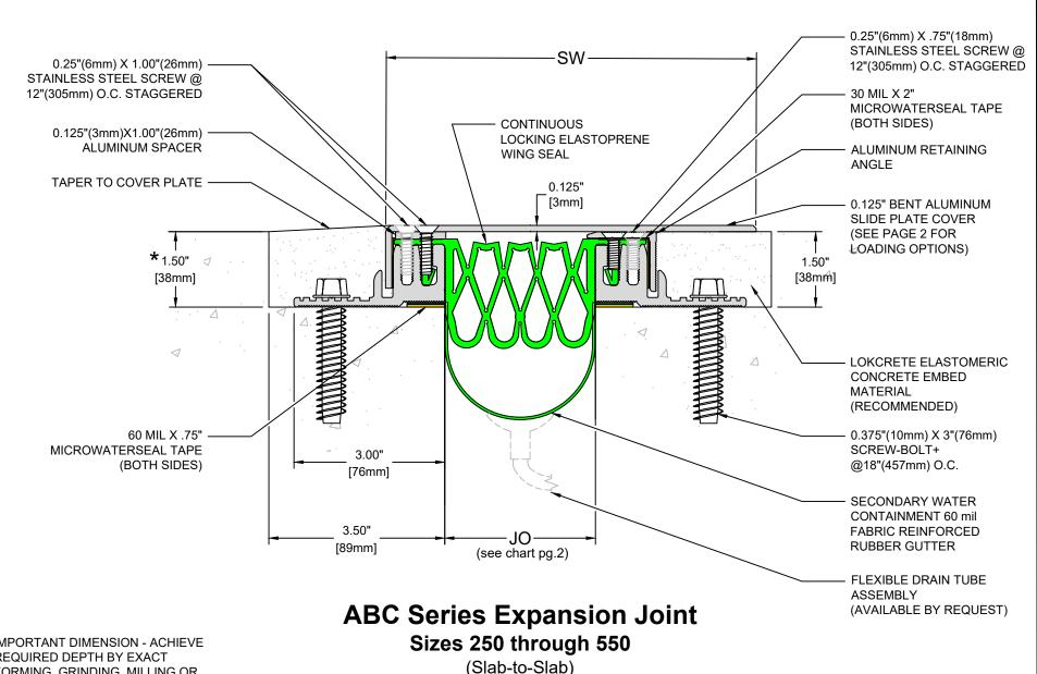
\*IMPORTANT DIMENSION - ACHIEVE REQUIRED DEPTH BY EXACT FORMING, GRINDING, MILLING OR STRUCTURAL LEVELING BED
