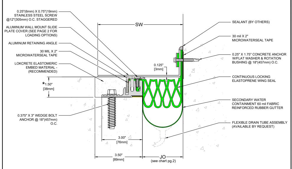
\* IMPORTANT DIMENSION - ACHIEVE REQUIRED DEPTH BY EXACT FORMING, GRINDING, MILLING OR STRUCTURAL LEVELING BED
