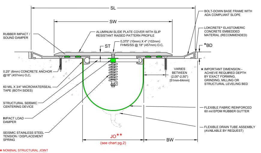
\* \* NOMINAL STRUCTURAL JOINT WIDTH INCREASED 3 INCHES TO ACCOMMODATE FULL **CLOSURE**
